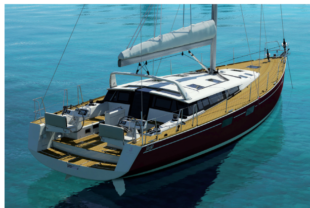
PACE SETTERS Left: The new Oceanis 48 features a 'centred' rig, hard bimini located mainsheet and optional Dock&Go Right: Motorboat style saloon with plenty of space and airiness characterises the Sense range.
