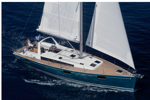
PACE SETTERS Left: The new Oceanis 48 features a 'centred' rig, hard bimini located mainsheet and optional Dock&Go Right: Motorboat style saloon with plenty of space and airiness characterises the Sense range.
