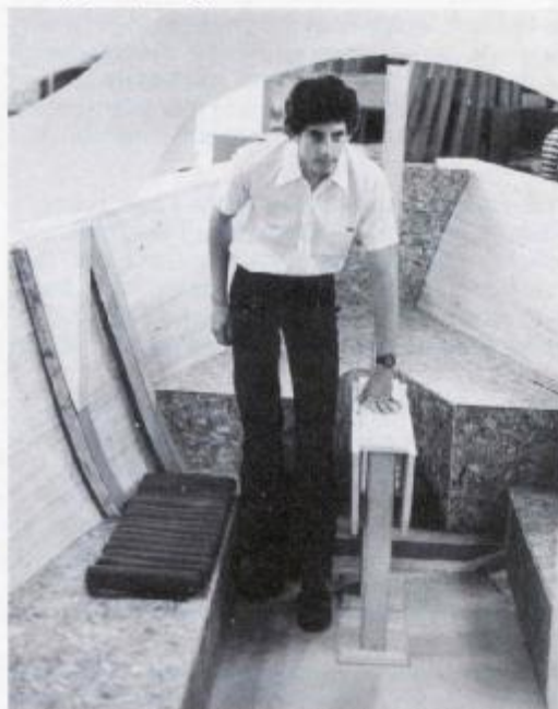
Full scale interior mock-ups were used to test over 12 different interior arrangements.
