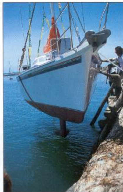
Out of the water the Phase 4 reveals a shallow draft fin keel with a highly efficient wing keel.
