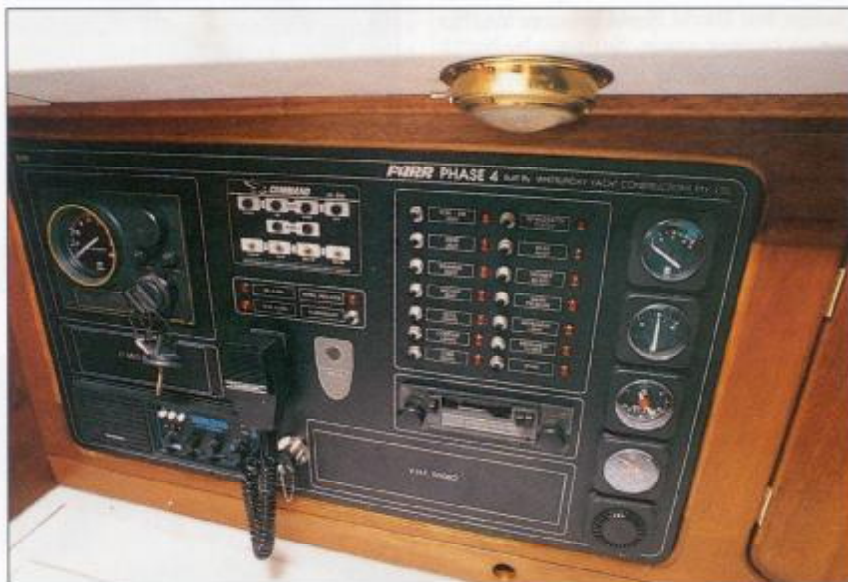
Purpose-made instrument panel groups all of the electrical systems into one sensible, easy-to-read console.
