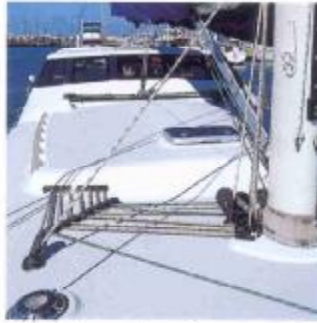
Halyards run from the mast under cabin top to the cockpit.
