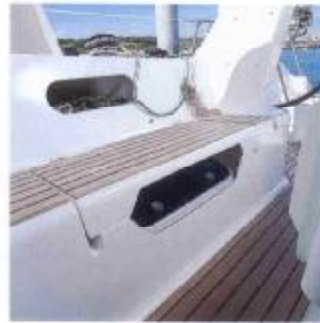
Opening ports give ventilation under closed hatches.
