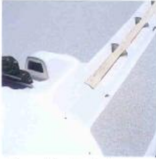
Recessed hand rail and air vent details.
