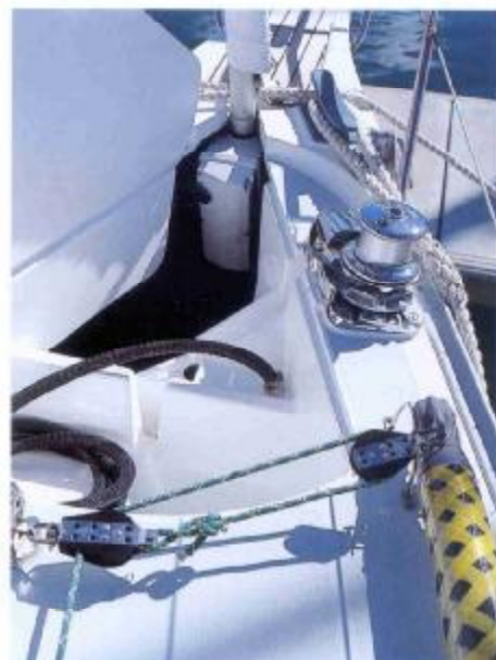
Anchor winch, chain and stowage locker and underdeck headsail furler.
