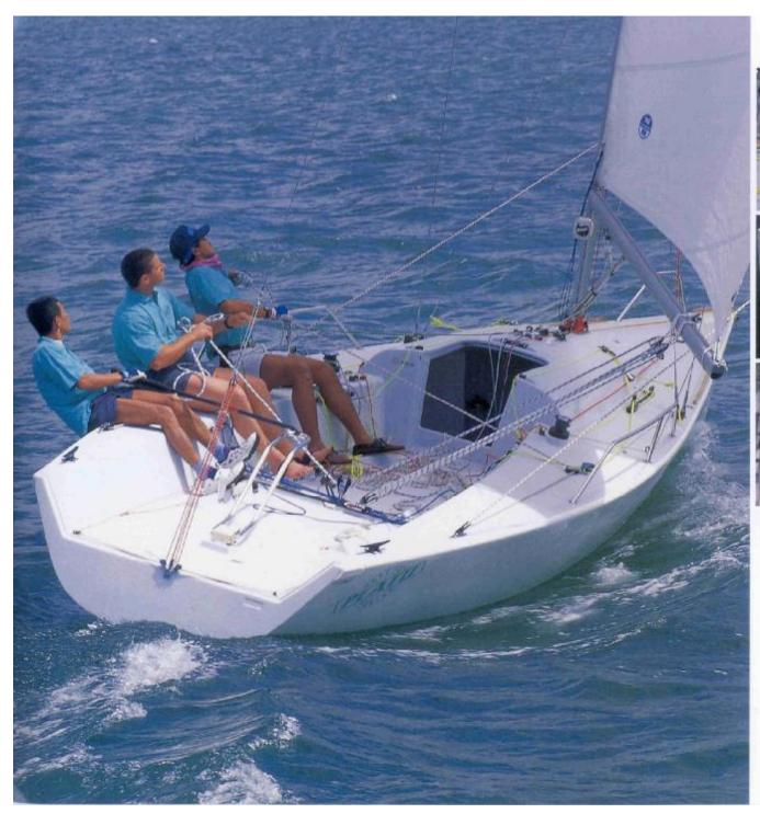
The rig is twin spreader, swept back configuration with discontinuous rigging featuring a Fosters anodised section.
