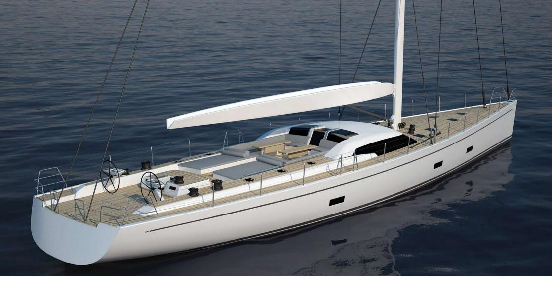
This project combines the successful lay-out already seen on the SW 100' with the advantage of a **more modern hull** with a remarkable gain in the water line lenght of 1.35 mt. This LWL increase offers significant **advantages while sailing in any condition** and even steaming, while the aft flatter hull bottom is a promise of **higher performances** and and increased stability especially in reaching conditions.
