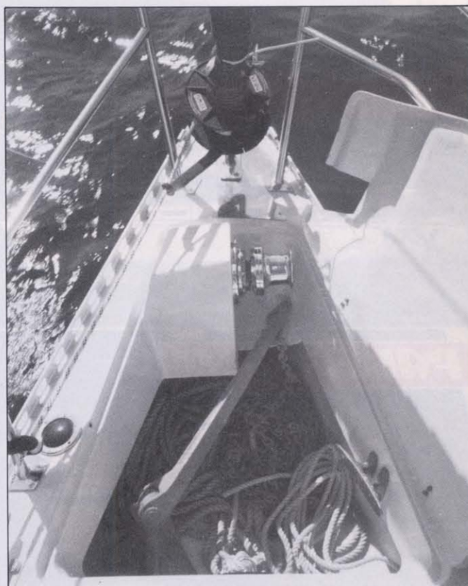
Anchor winch inside deep anchor locker.
