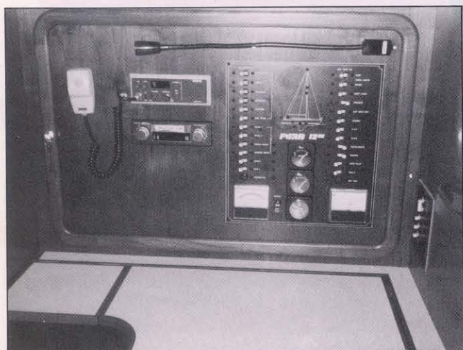
Comprehensive control panel over navigation table.
