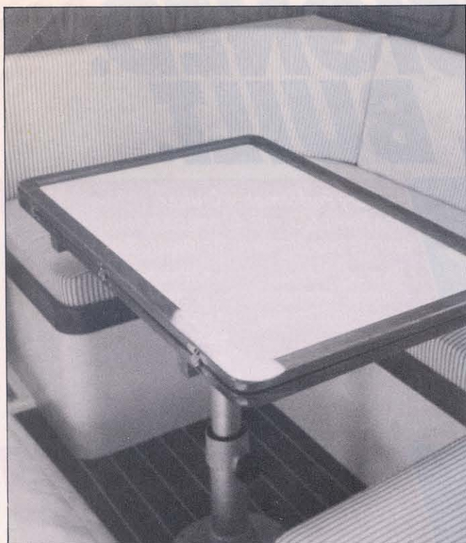
Dinette table can be dropped to form a double berth. Table opens to serve settee opposite.
