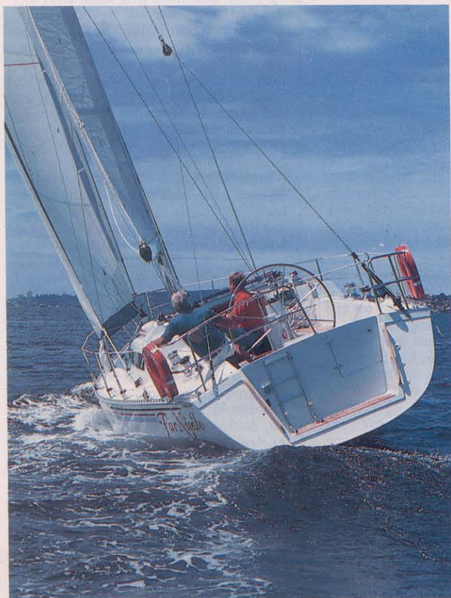
Boarding platform with walk-through door to cockpit is a feature of a practical and comfortable deck lay out.
