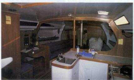
On this page: The interior arrangement is fairly sparse by cruising boat standards but positively sumptuous by modern race boat thinking. Looking forward from the galley the chainplate partial bulkhead can be seen behind the mandatory IMS full bulkhead. Looking aft from the mast the rows of bunks can be seen behind the galley, full standing headroom as befits a boat of this size
