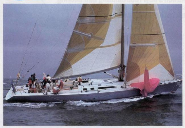
Above: Brindabella is designed for fast downwind sailing in the breeze. A masthead spinnaker hoist is fitted for downwind only races when a different IOR certificate must be used (see sailplan on page 68)
