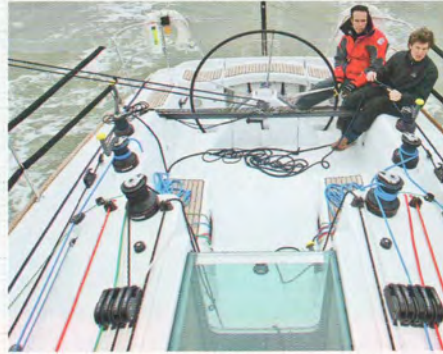
Left: Harken's Quattro winches allow fast spinnaker control. Right: the Bénéteau's spacious cockpit layout
