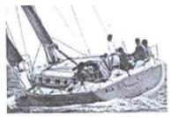
LOA 44'10"; LWL 37'8"; Beam 13'3"; Draft 7"1" (Standard), 8'8" (Optional); Displacement 20,126 lbs.; Ballast 8,047 lbs. (Standard), 7,518 lbs. (Optional); Sail Area 1,032 sq. ft.; SA/D 21.93; D/L 168; L/B 3.38; Auxiliary Volvo 2040; Fuel 57 gals.; Water 222 gals.
