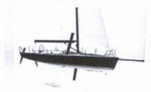
LOA 36'8"; LWL 32'10; Beam 11'3"; Draft 8'10"; Displacement 5,300 lbs.; Ballast 2,400 lbs.; Sail area 836 sq. ft.; SA/D 44; D/L 67.8; L/B 3.26, Auxiliary Yamaha 15-hp; Fuel 10 gals.
