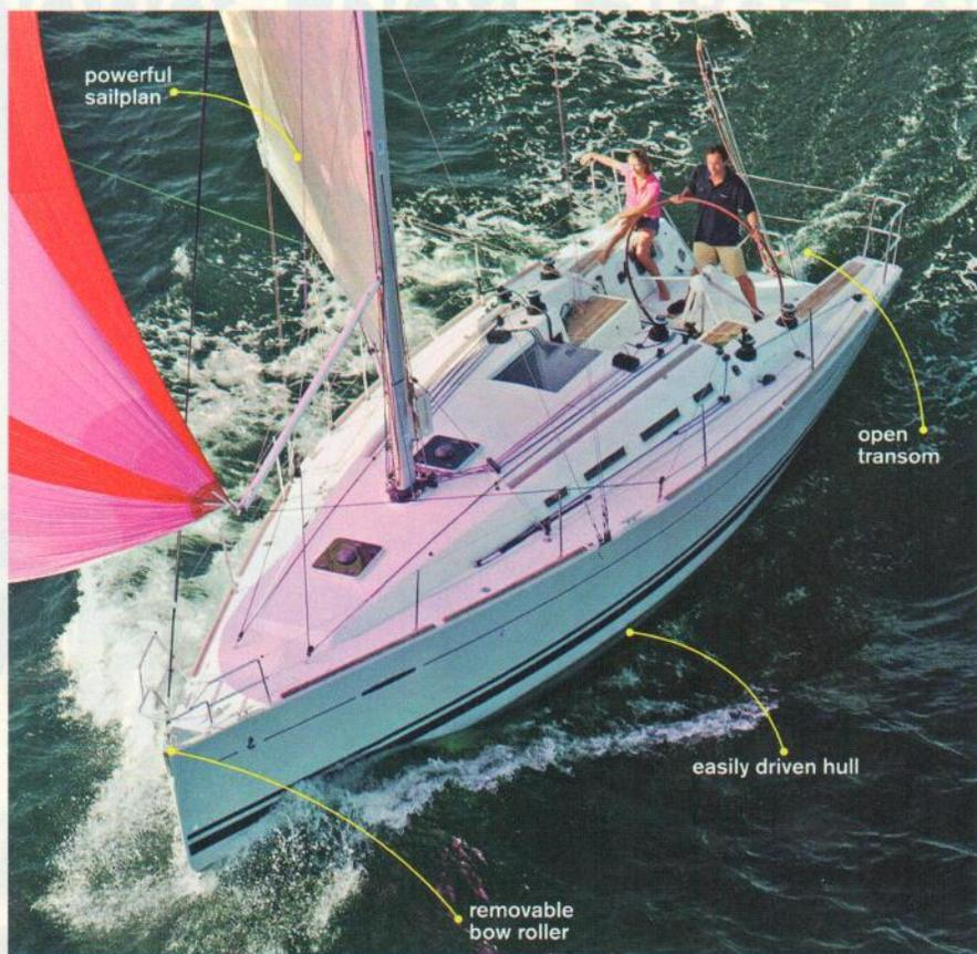
the boat. It can be closed off with a removable beam. There's reasonable storage in a large locker and in a lazarette below the sole, which could also take a liferaft.
