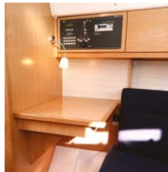
A small, aft-facing chart table is a function of the large heads compartment. T&G-style mouldings are used to line the hull sides
