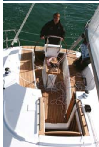
BELOW: The mainsheet is taken to a strong-point on the cockpit table and can just be reached from the helm. The space beneath the table is wasted; it could be used for stowage
