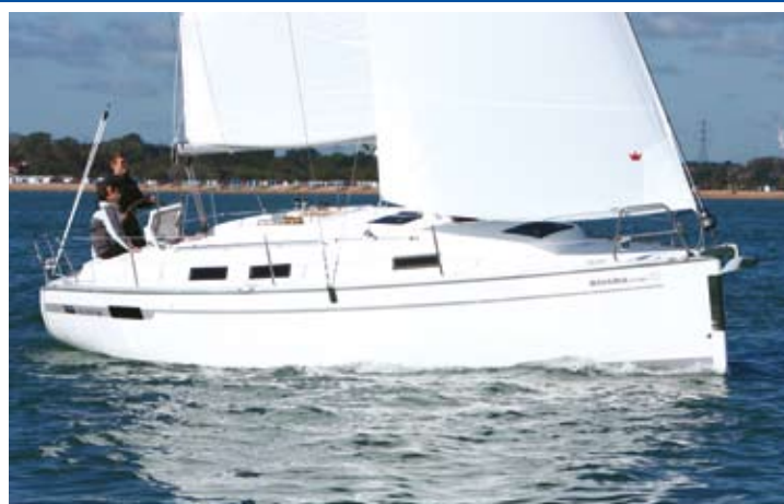
A rig with a minimal-overlap headsail is a new departure for Bavaria
