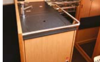
The galley is modest and with limited stowage. A stainless rail is easy to grab and simplifies cleaning but allows small items to slide off
