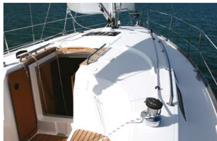
The flat, clear coachroof is easy to move around in when dry and upright, but the flush-fitting hatches and ineffective non-slip limit grip in the wet
