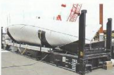
Above: the transport system developed for the Farr 400 mimics that used successfully by the RC44 fleet (left). A big square-head main makes twin backstays essential (far left), although the aft-swept shrouds give security for the carbon spar. The hull is a nice mix of low wetted surface rounded sections plus a moderate raised aft chine. Production boats feature a lateral grinder pedestal for easier use when heeled – the grinder also drives the keel-raise system
