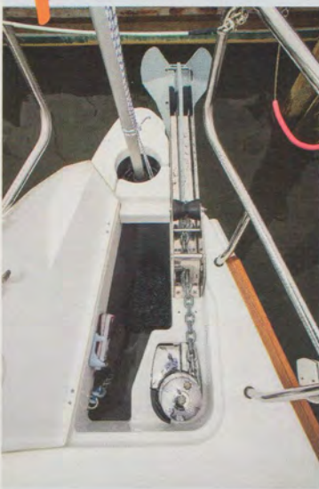
Hideaway The roller-furling unit for the genoa and the windlass for ground tackle are recessed in the foredeck.
