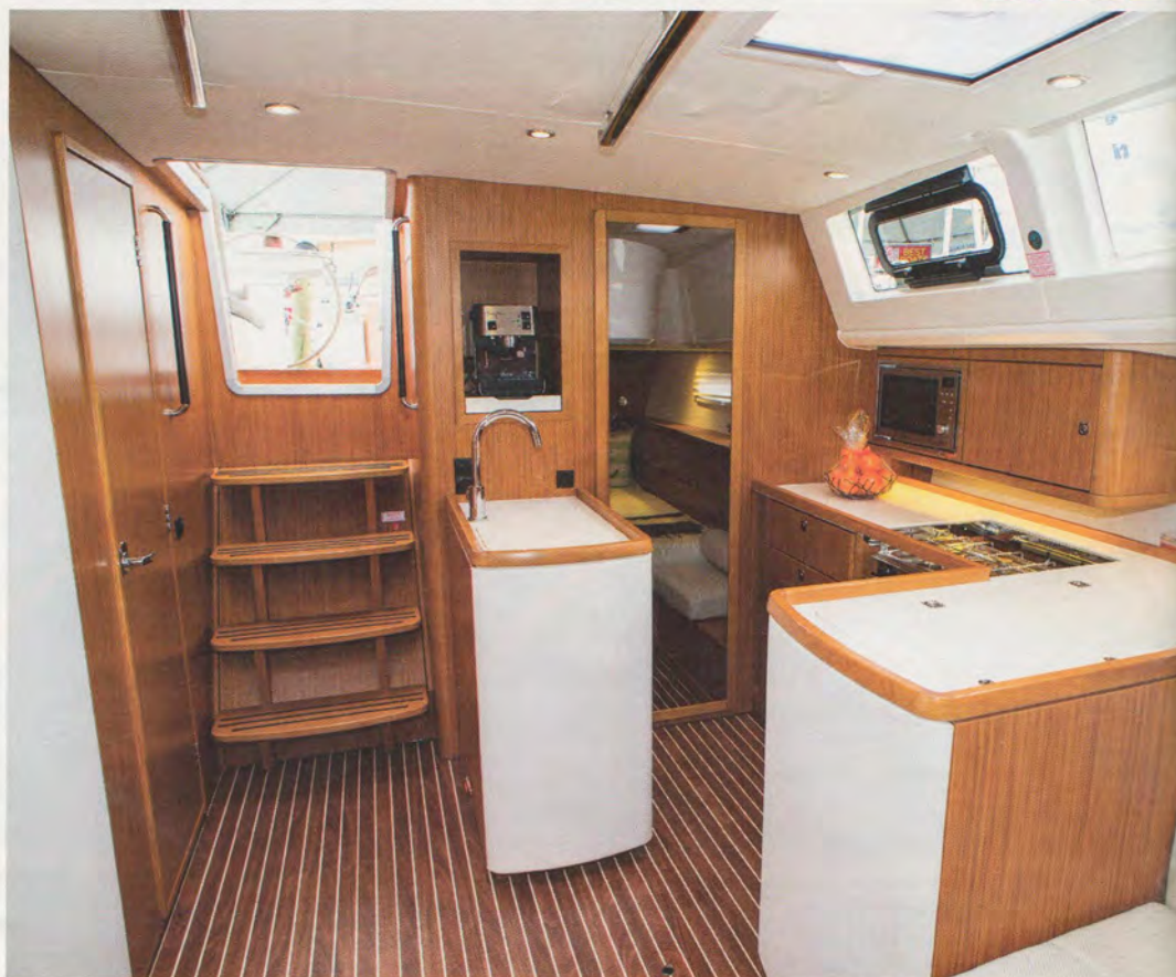
The deck saloon design makes for a bright and airy cabin. The companionway is offset to starboard, creating a large space for the galley.
