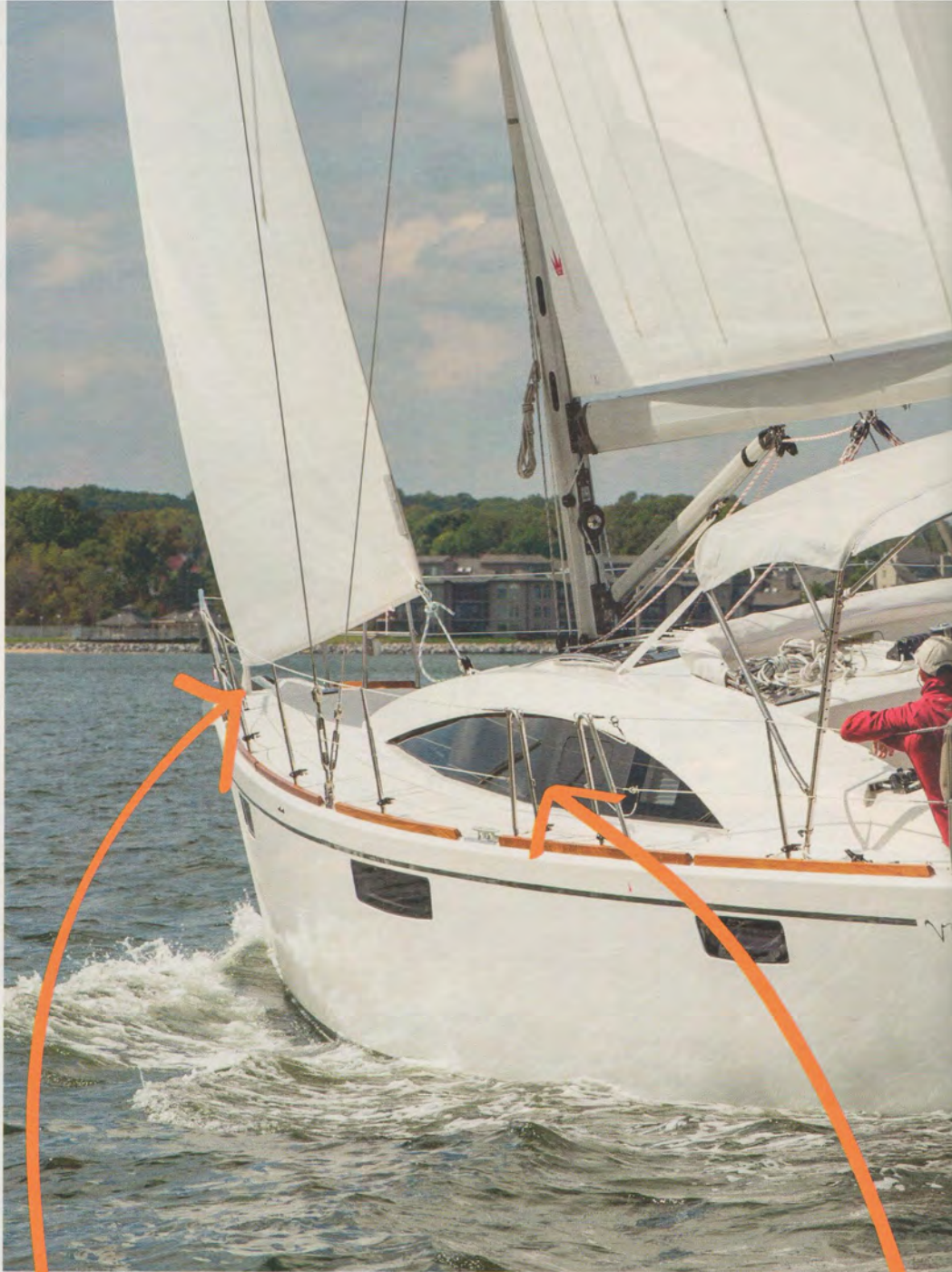
Hideaway The roller-furling unit for the genoa and the windlass for ground tackle are recessed in the foredeck.
