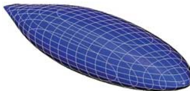
Above: the finalised VO65 bulb shape.
