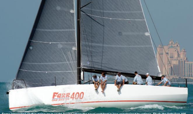
Some interesting stuff is going on in yacht design where the naval architect is less constrained by ratings. Study the light Farr 400... aft there is the family resemblance to recent VO70 and TP52 shapes, but melded onto the beginnings of a much fuller scow-type bow
